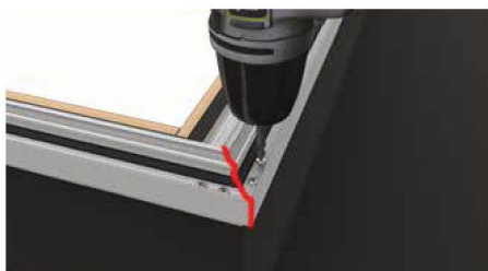
5 Using the 4.2 x 25mm screws provided, screw through the pre-drilled holes into the cleat to secure.
