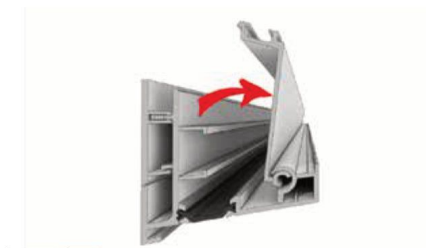
7 Insert ringbeam flaps by locating hinge part of the flap into the main ringbeam at approx 80 degrees as shown, then rotate forward to lock in.
